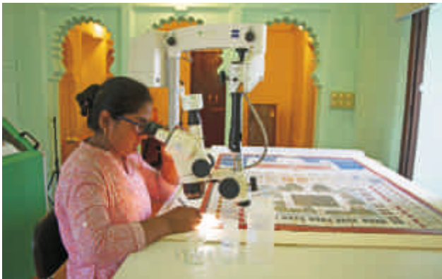
Consolidation of paint layer being carried out under stereo microscope
