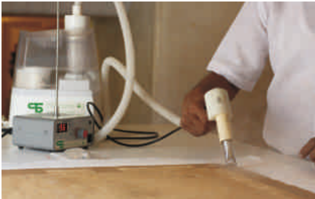
Use of steam pencil for removing old adhesive
